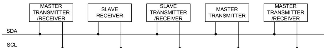
Figure. 5 System configuration
