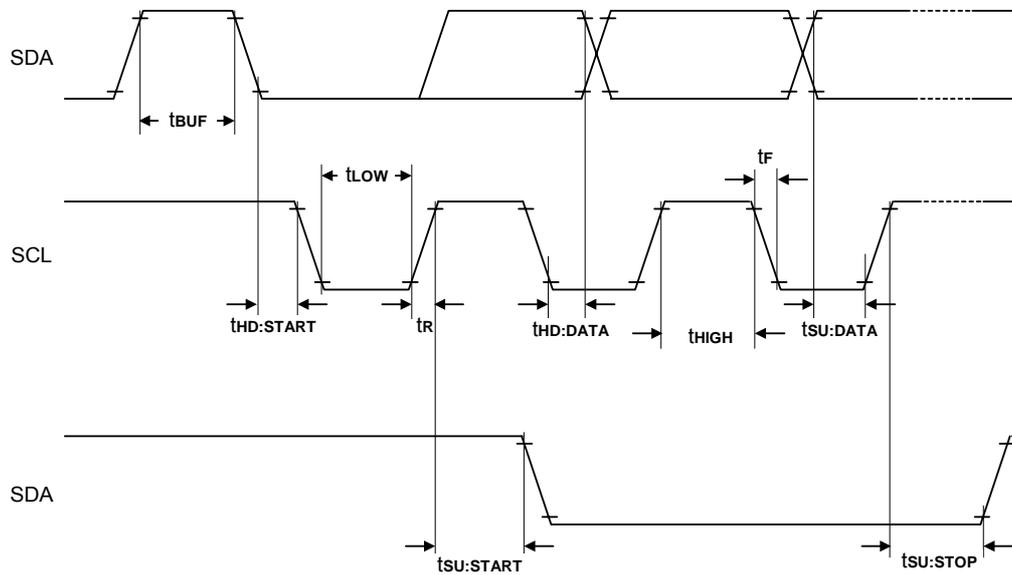
(V<sub>DD1</sub> = 1.65 - 3.5V, T<sub>A</sub> = +25°C)
